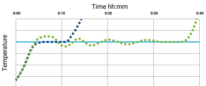
Without rocket controller: Long settling time to the target temperature
