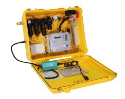
The 25 CFM three-stage filter system efficiently removes particulates, oil vapors and hydrocarbons from an air supply. After filtration, the regulator sets the pressure for the respiratory equipment and the manifold assembly provides two outlets for airline hose quick connections.
