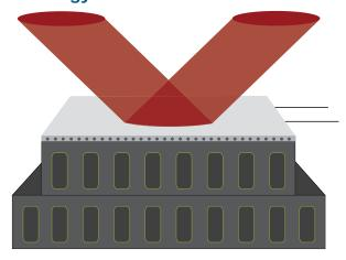
All chilled mirror sensors measure the actual temperature that moisture condenses to provide a reading of dew point. This fundamental technique gives unparalleled accuracy and reliability. Chilled mirror hygrometers are commonly used as secondary or transfer calibration standards for humidity.
