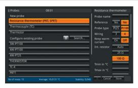
In this menu the probe settings can be selected and the reference thermometers can be stored under a unique name.
