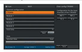
In this menu the user can define a scan by selecting the channels and the hold time. For activating the scan use the start button.
